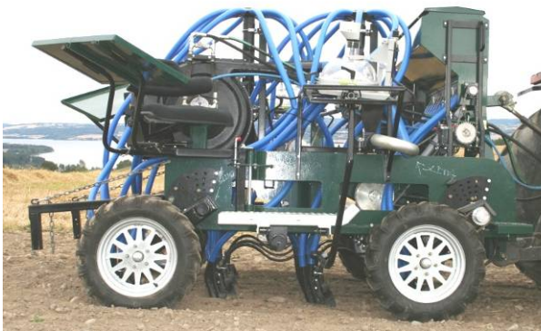
Smallaire components including venturii ( lower right) – note slim line of blower on plot machine – centre top blower has 150 mm outlet while the others have 75 mm outlets
