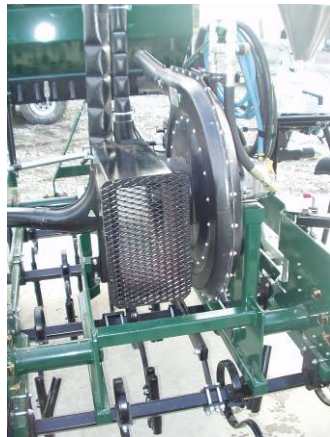
Smallaire components including venturii ( lower right) – note slim line of blower on plot machine – centre top blower has 150 mm outlet while the others have 75 mm outlets
