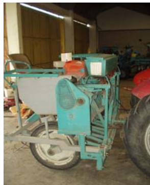
Locally manufactured Oyjord – Type plot seeder fitted with Duncan arable seed drill coulters to which forged interchangeable knock-on knife tips are fitted.
