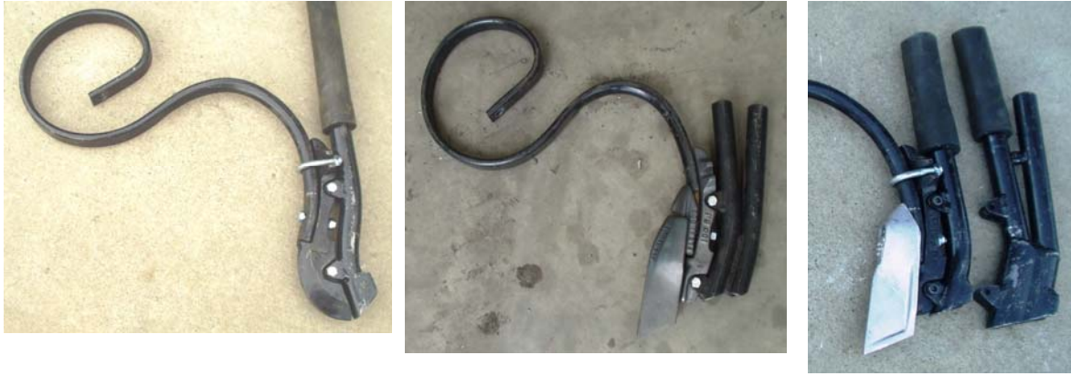
Plate 2. Available range and use of bolt-on and knock-on tips fitted to trailing hoe and 12mm S tynes, plus matching seed tube options. Suffolk shoe option is shown – for which a double seed hose is also available. All knock on tips are interchangeable using the same cleat.
